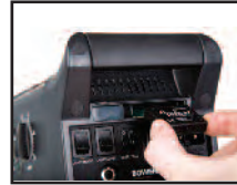
Insert Radio Trigger Card into slot and replace RF Module Cover.
