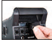
Plug in antenna into side of unit. Remove RF Module Cover.
